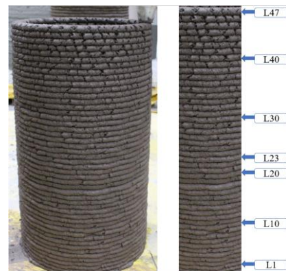
Figure 3 - Printed Element B (left), Section considered for analysis and the layer designations of Element B (right)
